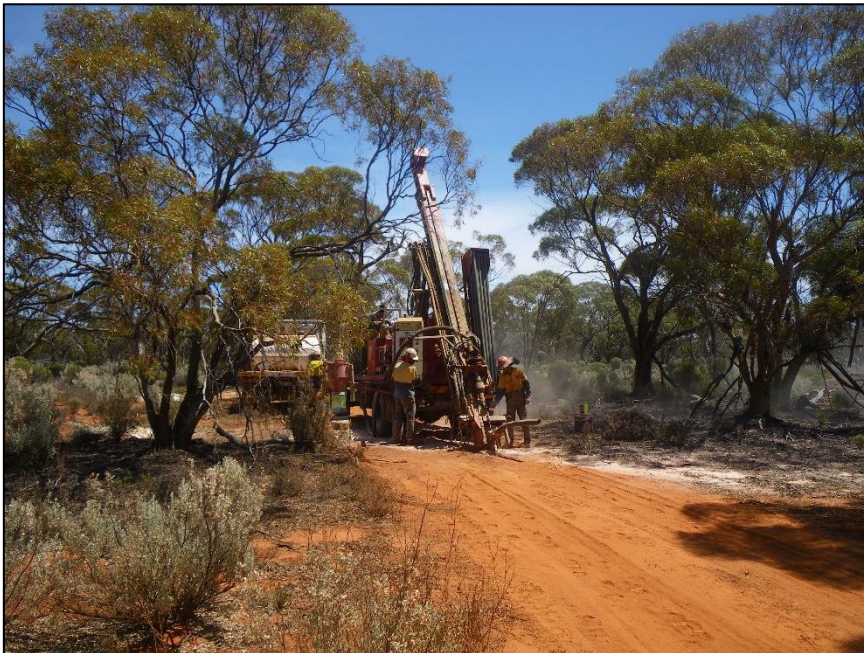
Figure 1: RC Drilling underway at Torian's Paradigm North Prospect.
